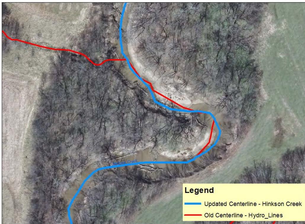
Figure 2. The centerline for Hinkson Creek was updated (blue) in places where 2007 line work (red) did not reflect stream conditions in 2011.
