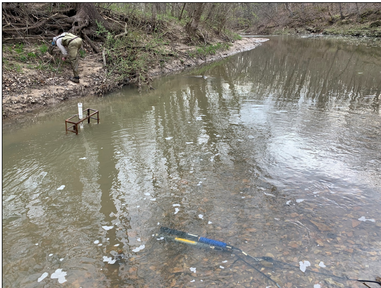
FIGURE 5. Hinkson Creek Site 7 Continuous Conductance Monitoring Instrumentation.
